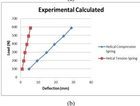
Figure 2:- Variation between load and Deflection for helical compression spring (a) Manually, (b) Experimentally
