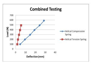
Figure 3-:-Variation between load and Deflection for helical compression spring
